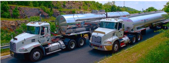
*Carbon Express has aluminum non-insulated trailers for both oils and solvents that allow us to maximize each load.*
